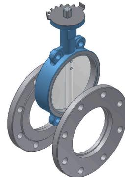
2. Insert four pairs of bolts /nuts gently into the flange hole and tighten the nuts to correct the plane degree of the flange face. Note this type valve does not require adding sealing gasket.
