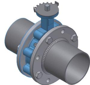
9. Open the valve to ensure the disc can opened and closed freedom.
