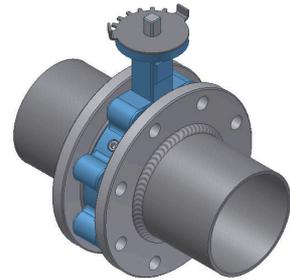
8. Correct the valve position and tighten the two face bolts in order of diagonal.
