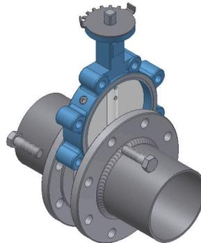
6. Fix the flange on the pipeline completely by welding. When welding, it should be uniform and fast, to prevent to product welding stress, cause the flange surface deformation. Ensure the two pieces of flanges are parallel and perpendicular.
