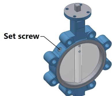
2. As shown in the figure, the valve is placed between two pieces of pre-installed flange. Note that the flanges should be parallel, flange surface should be flat, no burr and acute angle around the sealing surface, bolts holes should be aligned neatly.
