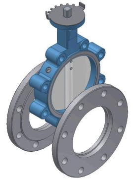
3. Using bolts fix the valve, (at least 4 bolts each face or more) to correct the plane degree of the flange face. Note this type valve does not require to add sealing gasket.
